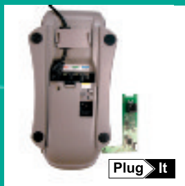
Modular architecture for SIMs and communication
